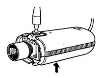
Note: Do not clamp the cable with this installation.
