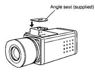
**Caution:** When the left and right pan limit screws should be removed from the pan/tilt unit due to the Angle-A installation, use the Angle Sheet as shown below.
