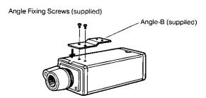
b-3. Re-install the mounting adaptor on the Angle-B.
